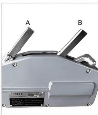
4. Hand operated forward handle A, the wire rope can move forward
